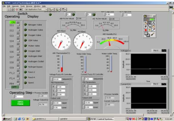
Figure 6: Control interface of the PEMFC system
