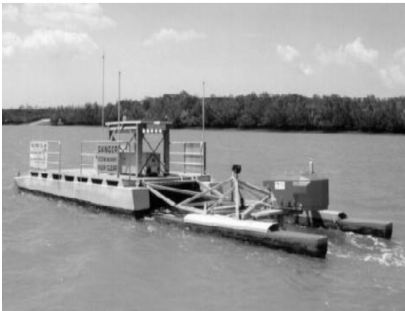
The Tidal Power Unit in the Apsley Strait
