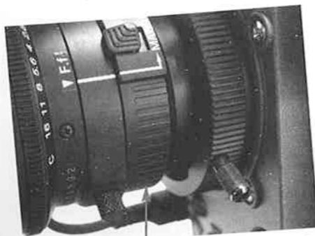
You adjust focus in macro by turning the macro ring.
