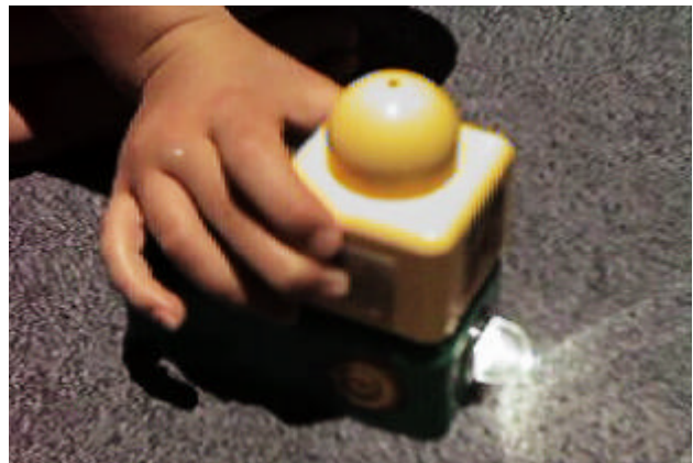
Figure 2: A touch block attached to a light block will cause the light to turn on whenever sensor plate is touched.
