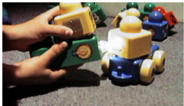
Figure 3: A remote control car demonstrates interaction between block stacks. The touch block on the light block forms the remote control for the car formed by placing a seeing block on a movement block.
