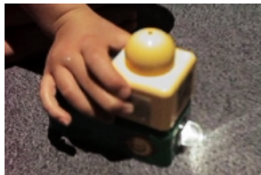
Figure 1: A touch block attached to a light block will cause the light to turn on whenever sensor plate is touched.
