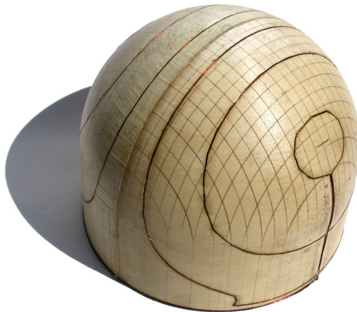
Figure 8. The half-scale prototype shielded X gradient coil.
