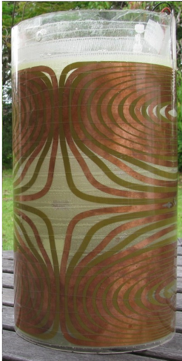
Figure 1: Photograph of the \min(P) prototype coil with N_c = 20 before painting.
